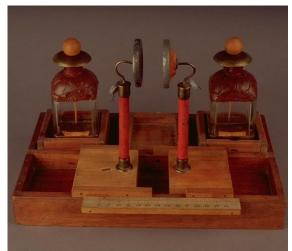
1837 – the influence of different insulators in determining the capacitance to store electrical charge in an equipment is quantitatively measured by Faraday. The SI measure unit of capacitance is the Farad (one Coulomb per Volt).
