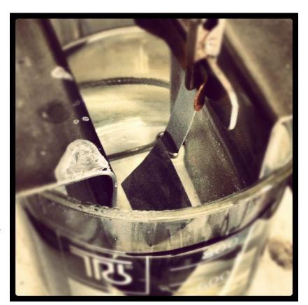
Capacitance dependence on surface and distance (and electrolyte) makes the rolling operation a very delicate step when building a capacitor.
