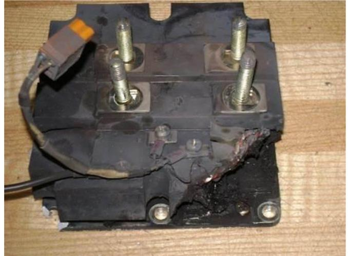
Figure [1] – Example of a failed IGBT
