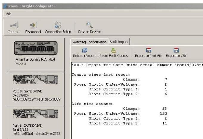
Figure [4] – Example of Fault Reporting in Amantys Power Insight Configurator
